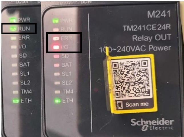
Figure A1: PLC State Changes
