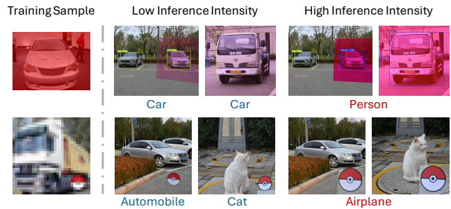
Figure 10: Blended (top) and BadNets (bottom) attacks in the physical domain: attacks can succeed only when inference-phase trigger intensities are higher than training-phase intensities (larger size or higher opacity).
