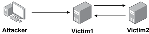
Figure 5: Ping-Pong Amplification Attack . The attacker sends the encapsulated packet to the first victim, who will decapsulate the header and forward it to the second victim. This continues until there are no more headers in the datagram.
