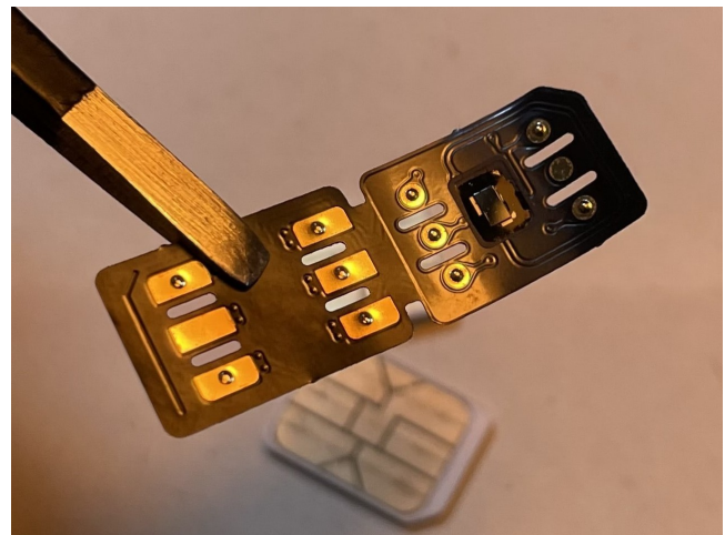
Figure 10: An interposer; a very thin, flexible smart card with contacts on both sides. It is typically placed between a SIM and the phone to intercept and rewrite communications.
