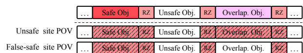
Figure 3: RUSTSAN’s shadow memory coloring scheme. Safe objects are colored with magenta , overlapping objects with pink , and unsafe objects are non-colored.
