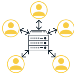
Figure 1: Illustration of FL in centralized setting: model parameters are sent back and forth between a server and clients.
