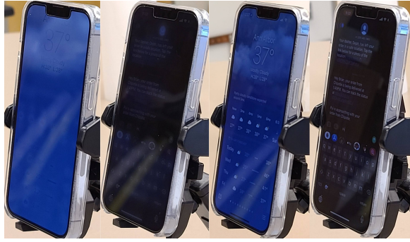
Figure 5: Photos of screens protected by Eye-Shield (left) and the unprotected original screens (right). Photos were taken at a distance of 19.7” and an angle of 45°, from the perspective of a shoulder surfer. The images were captured with a 108MP, f/1.8 , 26mm smartphone camera at 3\times zoom.
