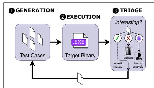
Figure 1: A visualization of software fuzzing’s fundamental steps.
