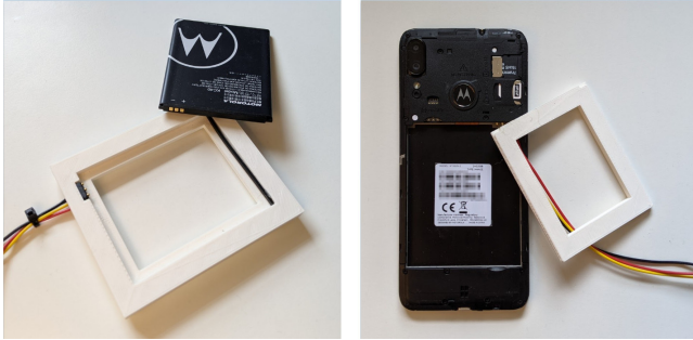
Figure 14: Photographs showing the 3D printed battery holder and inlet.
