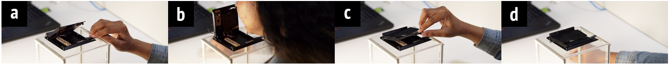
Figure 3: When unmuting Candid Mic , (a) a user presses a lever to open the cover of Candid Mic , and (b) says voice commands once the cover is open. (c-d) Otherwise, the user can manually close the cover.
