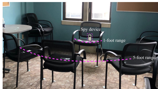
Figure 4: Our experimental setup. We created nine total equal-height place markers at 1 foot, 5 feet, and 10 feet away from a spy device and recorded each detector’s reading at each place marker. The 10 foot place markers are not shown.
