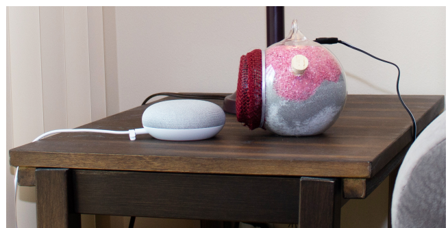
Figure 1: The Obfuscator design probe next to a Google Home Mini Device. Obfuscator uses ultrasound jamming to prevent the smart speaker from listening to the user’s conversations and is designed to appear as a tabletop “trinket” to blend into the user’s home environment.
