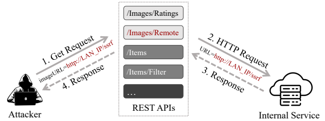
Figure 2: Exploitation process of CVE-2021-29490.
