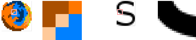
Figure 8: Pixel-based content continues to stay pixelated after stretching (Left), whereas vector-based content is re-sampled after stretching (Right). Both regions in the original images are the same 3 \times 3 px size.
