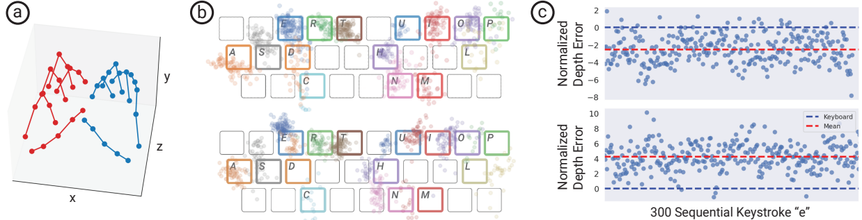
Figure 4: (a) A sample instance of H_{org} where the left pinky is pressing a key. (b) VR collected (x, z) touchpoints from 2 participants. The corresponding ground truth key positions are marked with the same color. Top-15 frequent letter samples are shown. (c) Depth of sequential keystrokes when ‘e’ is typed by Participants 1 and 2. Normalized depth error puts the ground truth at zero and scales by the height of an individual key. Standard Deviation for Participant 1: 1.639. Standard Deviation for Participant 2: 1.853.
