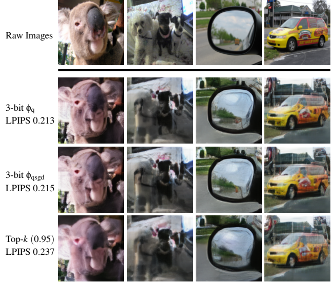
Figure 6: Reconstructed images when gradient compression is applied in FedAvg. The compression methods include: 3-bit uniform quantizer \phi_q , 3-bit QSGD quantizer \phi_{\text{qsgd}} , and Top- k method \phi_{\text{topk}} with the sparsity set to 0.95. The reconstructed images are visually similar to the raw private images.
