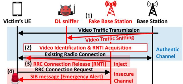
Figure 11: End-to-End attack procedure
