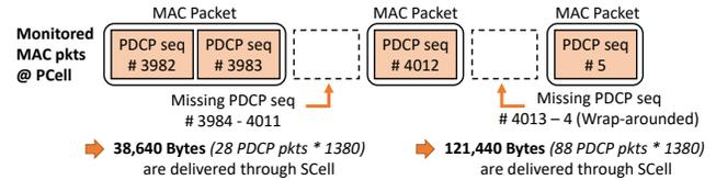
Figure 5: Example of estimating lost traffic volume in CA
