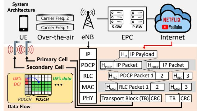
Figure 1: LTE network architecture and protocol stack
