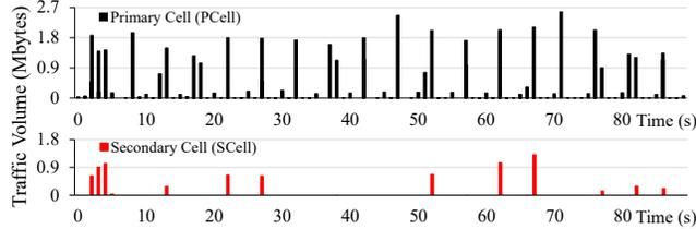
Figure 3: UE’s streamed video volume using 2-band CA
