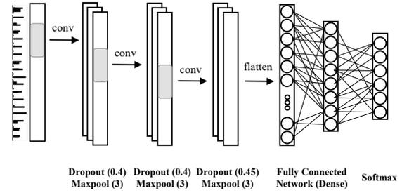
Figure 6: The structure of the used CNN model
