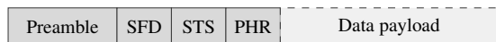
Figure 4: Example format of an HRP packet [4]. The field lengths and their order depend on the configuration.
