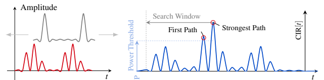
Figure 3: The CIR is calculated based on the received signal and a local template of the expected signal. A correlation peak indicates high similarity. However, with multi-path effects, there are multiple peaks. The receiver identifies the first LoS path, e.g., by searching back in time from the strongest peak.
