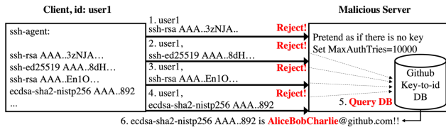
(b) Attack 1: Client De-anonymization. A malicious server rejects all of the client's public-key advertisement. This causes the client to advertise all of its public keys, under the default client behavior. The server can then use a key-to-id database to identify pseudonyms of the client, e.g., their Github username.
