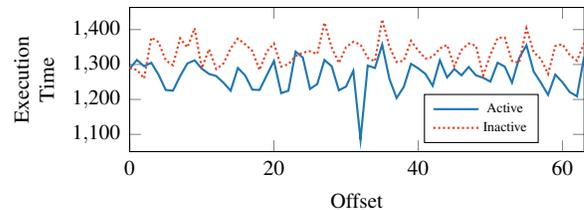
Figure 7: Template attack for page candidates of a kernel driver while triggering a supported `ioctl` syscall. The spike correlates with the kernel page containing the corresponding function, allowing to derandomize FGKASLR.
