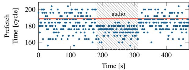
Figure 8: Detecting Bluetooth audio transmission with TLB-Evict+Prefetch. After 180 s, a 2:10 min song is played. Dots below the red line indicate that the page is in the TLB, *i.e.*, active, dots above the line indicate that the page is not in the TLB. During audio transmission, the page is always active.
