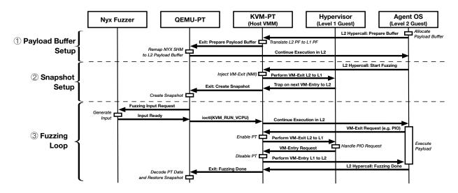
Figure 3: Overview of NYX's hypercall interaction between the various components: fuzzing logic, QEMU-PT, KVM-PT, L1 guest, and agent OS.
