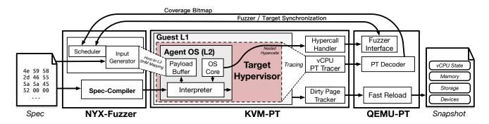
Figure 1: Overview of NYX's architecture. The architecture consists of three main components: (i) NYX's novel fuzzing engine, (ii) a highly modified version of KVM-PT which enables nested hypercall communication and hypervisor fuzzing, and (iii) a modified version of QEMU-PT to support fast snapshot reloads.
