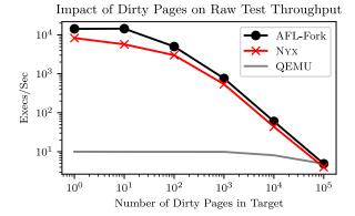
Figure 6: Comparing raw executions per second for targets that dirty *N* pages, with an AFL forkserver, QEMU's loadvm snapshot restore functionality, and NYX's fast full-system reloads.
