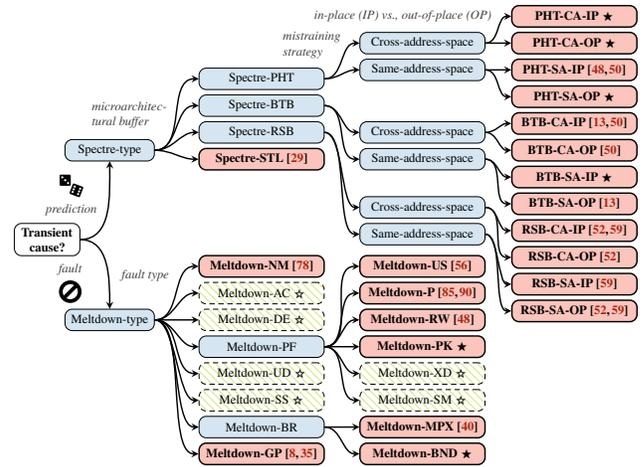
Figure 1: Transient execution attack classification tree with demonstrated attacks (red, bold), negative results (green, dashed), some first explored in this work (★ / ☆).<sup>2</sup>
