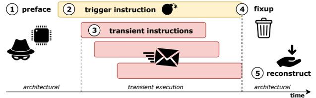
Figure 2: High-level overview of a transient execution attack in 5 phases: (1) prepare microarchitecture, (2) execute a *trigger instruction*, (3) *transient instructions* encode unauthorized data through a microarchitectural covert channel, (4) CPU retires trigger instruction and flushes transient instructions, (5) reconstruct secret from microarchitectural state.
