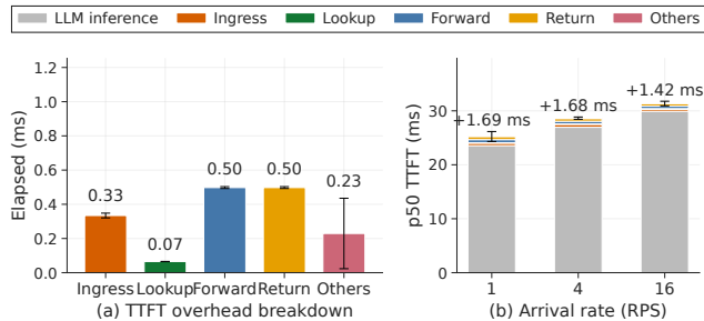
Figure 5: Control plane overhead of OpenTela. (a) Per-stage cost for a single request. (b) p50 TTFT decomposition at arrival rates of 1, 4, and 16 RPS with 256 input tokens.
