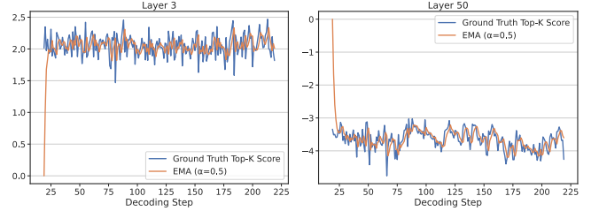
Figure 7: The 2048-th highest index scores in layers 3 and 50 of DeepSeek-V3.2 and prediction using EMA with \alpha = 0.5 during decoding.
