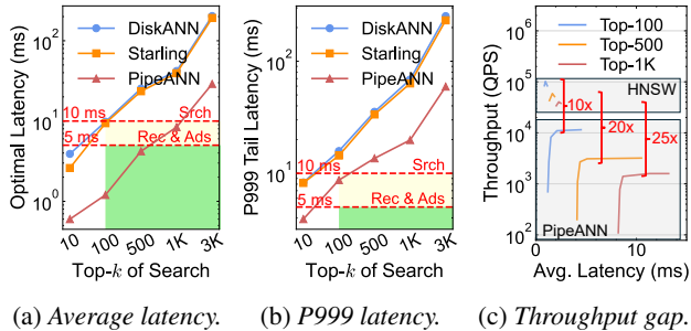
Figure 4: All graph-based systems fail in replacing in-DRAM solution. DiskANN and Starling can never meet the latency SLAs. PipeANN shows an insuperable gap in throughput. Srch refers to the search business, with latency SLAs of 10 ms. And Rec & Ads refers to the recommendation and advertising, with latency SLAs of 5 ms.
