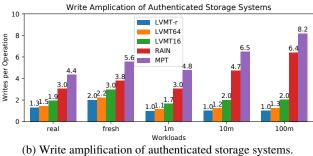
Figure 5: Read and write amplifications of authenticated storage systems.
