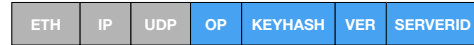
Figure 2: Pegasus packet format. The Pegasus application-layer header is embedded in the UDP payload. OP is the request or reply type. KEYHASH contains the hash value of the key. VER is an object version number. SERVERID contains a unique server identifier.
