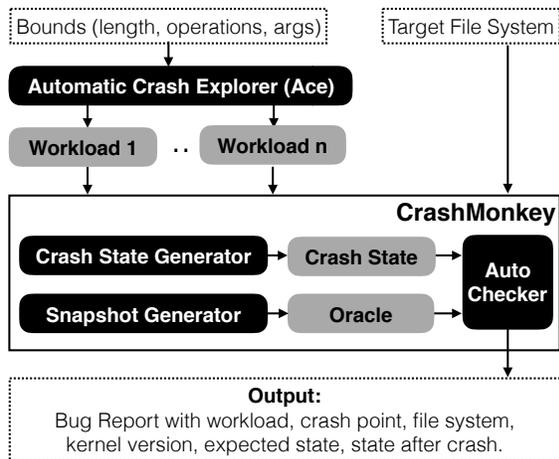
Figure 2: **System architecture.** Given bounds for exploration, ACE generates a set of workloads. Each workload is then fed to CRASHMONKEY, which generates a set of crash states and corresponding oracles. The AutoChecker compares persisted files in each oracle/crash state pair; a mismatch indicates a bug.
