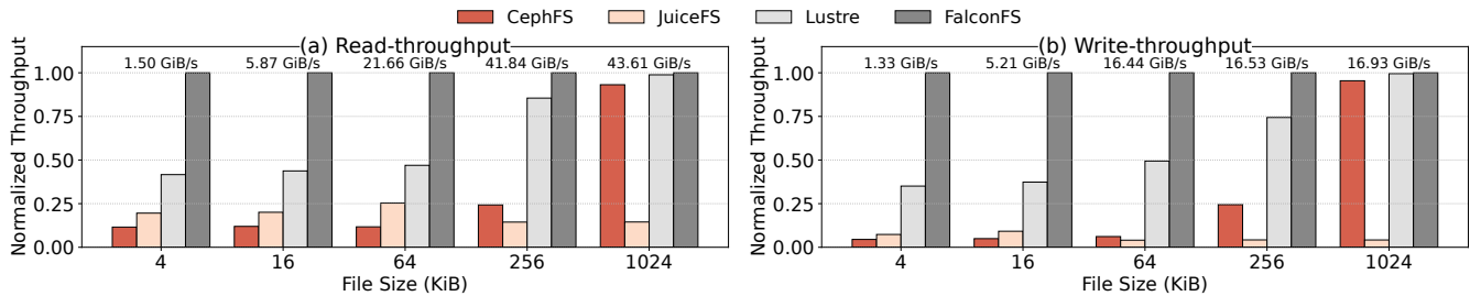
Fig. 13: Throughput of file data IO. Y-axis is the throughput normalized to that of FalconFS.
