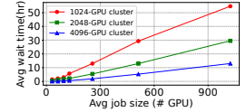
Figure 14: Avg job size vs Avg waiting time in the queue for different sizes of training clusters
