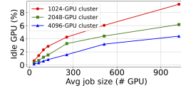
Figure 13: Avg job size vs Idle GPU for different sizes of training clusters
