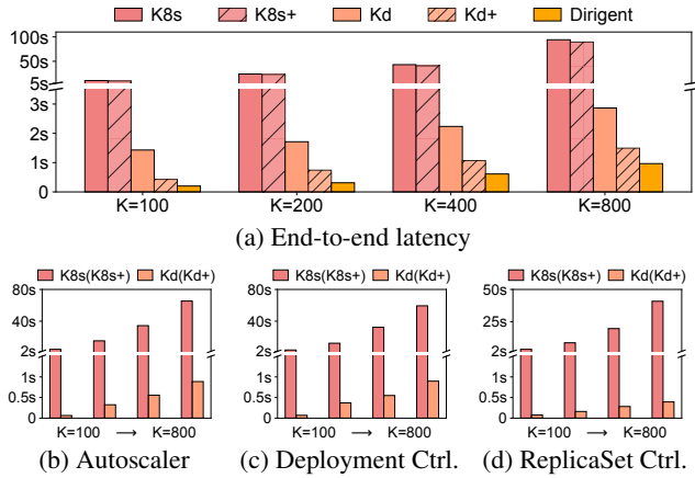
Figure 10: Upscaling latency for varying # of functions.
