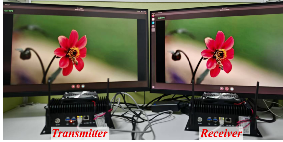
Figure 7: Showing Devices Used in System Prototype. Two NVIDIA Jetson serve as transmitter and receiver connected via network cable for end-to-end transmission.
