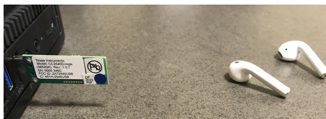
Figure 1: BBC enables direct communication between BLE chips and Bluetooth-Classic headphones
