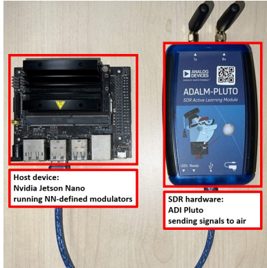
Figure 14: Prototype of NN-defined modulator. Left box: Nvidia Jetson Nano as the host device for the NN-defined modulator. Right box: ADI Pluto SDR as SDR hardware.
