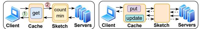
Figure 3: In-switch key-value store cache implemented using SwitchVM. ① and ② show the flow of cache hit and miss respectively. Cache-get/put/update and count-min represent DPFs and the pipeline they are executed on.
