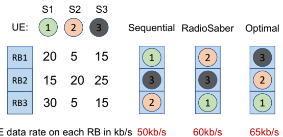
Figure 4: Allocating three RBs to three slices with same weights using different strategies.
