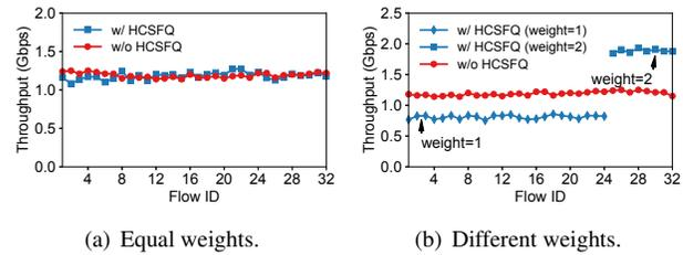
Figure 8: Testbed experiments of fair queuing for TCP.
