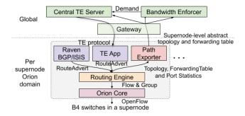
Figure 7: B4 Control Diagram
