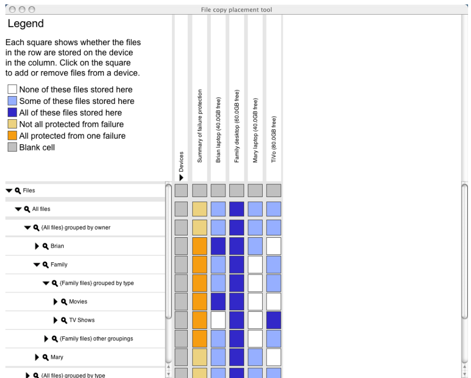
FIGURE 1: A SCREEN SHOT OF THE VIEW MANAGER GUI. ON THE LEFT ARE FILES, GROUPED USING FACETED METADATA. ACROSS THE TOP ARE DEVICES. EACH SQUARE SHOWS WHETHER THE FILES IN THE ROW ARE STORED ON THE DEVICE IN THE COLUMN.
