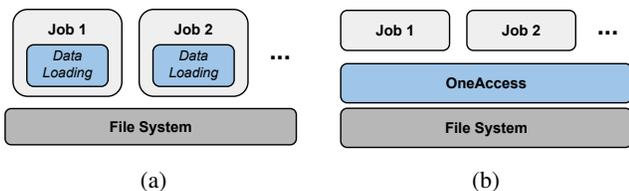
Figure 1: **OneAccess: A unified data loading layer for machine learning.** In (a), we show the design of current systems with standalone data loading; we’re proposing a dedicated data loading layer in (b).
