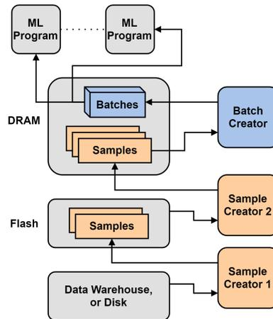
Figure 4: The architecture of OneAccess. The Sample Creator1 process generates reservoir samples from data on disk, and stores them on SSD. These samples are consumed by Sample Creator 2, which creates smaller reservoir samples held in memory. The Batch Creator process consumes the samples in DRAM to generate batches used by multiple jobs.
