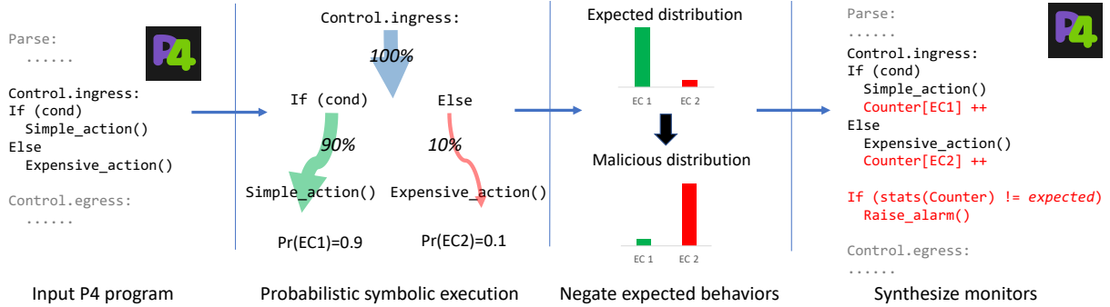
Figure 1: The workflow of our approach. Our engine a) takes in a data plane program written in P4, b) performs probabilistic symbolic execution to analyze common-case behaviors, c) automatically generates input traces that would trigger corner-case behaviors, and d) synthesizes a set of monitors to detect malicious patterns, and patch the original data plane system with them.
