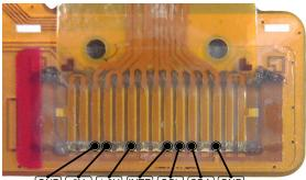
(b) The connection between the touch controller daughter board and the main touchscreen assembly daughter board of an assembly for the Nexus 6P. Marked: relevant pinout for the communication bus.
