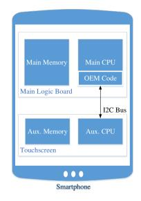
Figure 1: The smartphone, its touch screen, and its associated device driver software.
