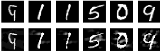
Figure 1: Adversarial examples for color depth reduction (to 1 bit) on MNIST. First row: original images. Second row: adversarially perturbed. Distortions, from left to right: 1.49, 2.61, 2.63, 3.83, 3.89, 3.90.
