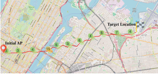
Figure 8: The hop-by-hop trace from Times Square, New York City, to a market near LaGuardia Airport (the number in each circle indicates the hop count in that area).
