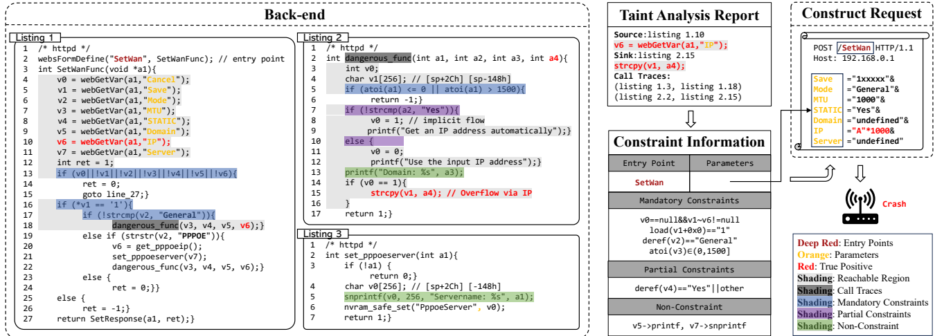
Figure 1: A vulnerability warning produced by EmTaint [6]. The example illustrates how a crafted input—guided by entry point inference and constraint modeling—can trigger a buffer overflow.
