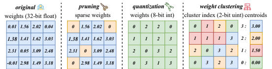
Figure 10: The same weight matrix subjected to pruning, quantization and weight clustering separately.
