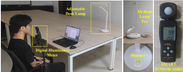
Figure 18: Testbed for investigation of ambient light.
