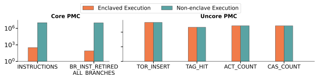
Figure 2: Core PMC and uncore PMC event counts when running microbenchmarks both in a production-mode enclave and in a non-enclave environment.
