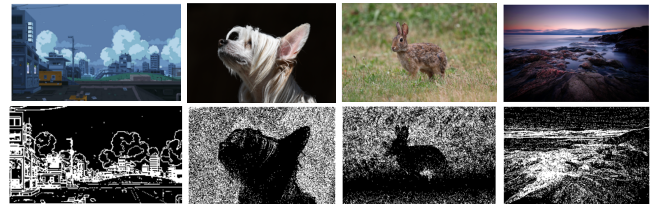
Figure 9: Original JPEG pictures (top) and their corresponding reconstructions from UncoreBleed (bottom). From left to right, the image resolutions are (1) 900 \times 600 , (2) 2160 \times 1280 , (3) 4016 \times 2016 , and (4) 6016 \times 4016 pixels.
