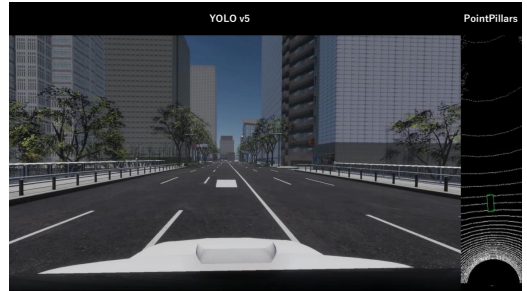
Figure 26: Detection results in the attacked scenario. PointPillars detects a non-existent car.
