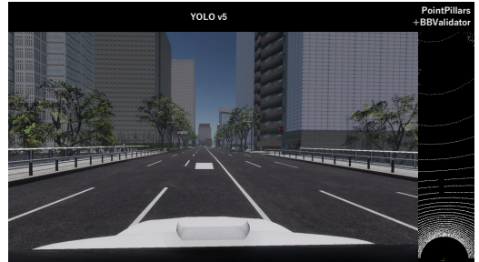
Figure 27: Detection results in the attacked scenario. PointPillars + BBValidator does not detect the non-existent car.
