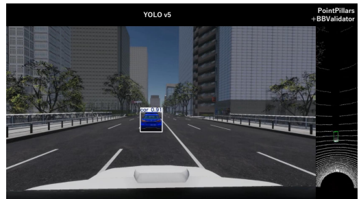
Figure 28: Detection results in the non-attacked scenario. Both YOLOv5 and PointPillars + BBValidator successfully detect the vehicle in front.
