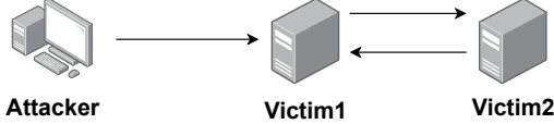
Figure 5: Ping-Pong Amplification Attack . The attacker sends the encapsulated packet to the first victim, who will decapsulate the header and forward it to the second victim. This continues until there are no more headers in the datagram.
